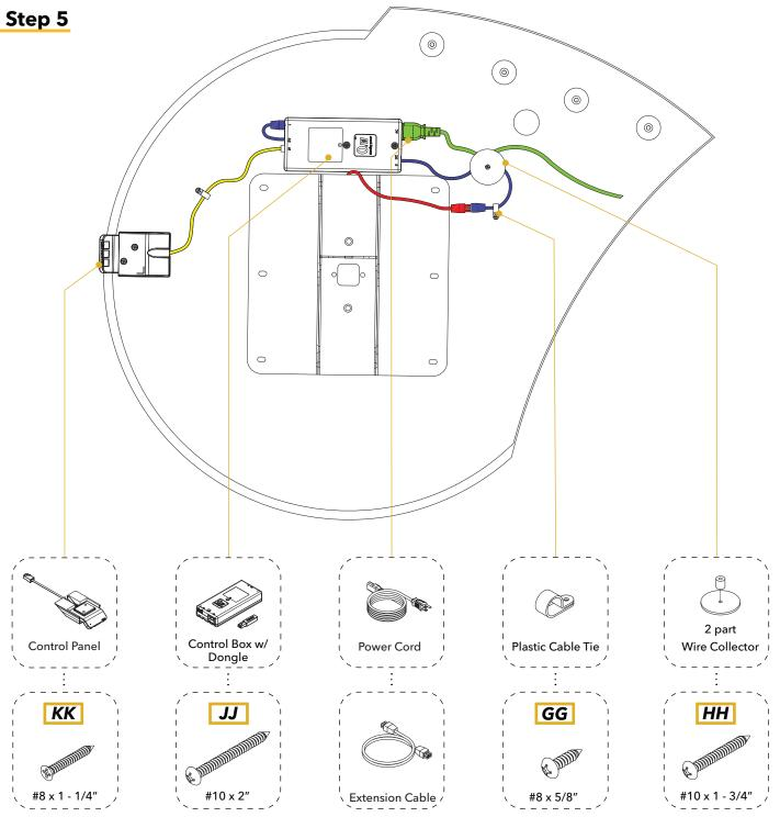
Line up Wire Collector collar and backing plate (2 pieces) and fasten to the countertop in the position shown using the [HH] screw. Route the Extension Cable (shown in blue) through the channel on the Control Box. Fasten the Control Box to the countertop, in the position shown using the [JJ] screws. Fasten the Control Panel to the countertop, in the position shown using the [KK] screws. Place the Plastic Cable Ties onto the wires as you route them and attach using [GG] screws, as shown.
